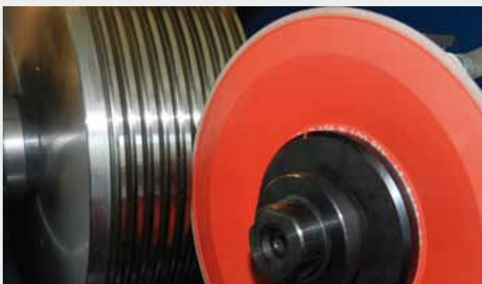
Bottom knives and multi-groove blocks grinding
